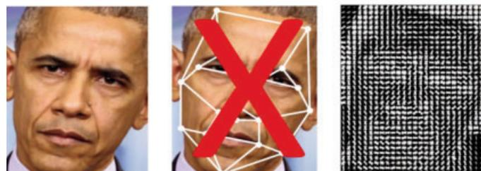
The new generation of solutions utilise the Histogram of Oriented Gradients (HOG) method. The solution generates metadata directly from the facial data via a Convolutional Neural Network (CNN), producing a data-string not unlike a DNA signature.
